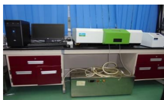
15. High Precision Dilatometer (NETZSCH Technologies, Germany) (Make: NETZSCH Technologies, Germany )
