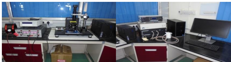
17. Precision Multiferroic Test System ( P-E , piezoelectric, pyroelectric, magneto-electric for bulk and thin-films) with temperature variation facility (Make: Radiant Technologies Inc., USA)
