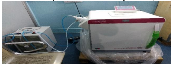
23. Microwave assisted Hydrothermal technique for nanomaterial synthesis (Milestone, Italy)
