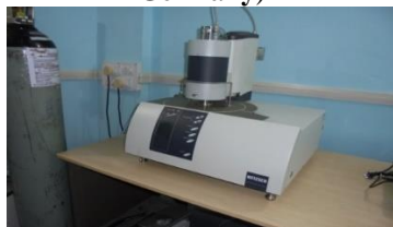
14. High Temperature ( lq. N_2 - 1600°C) Simultaneous TG-DTA / DSC Analyser (Make: NETZSCH Technologies, Germany )
