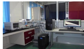
16. Impedance Analyser (40 Hz – 110 MHz) with temperature (up to 1000°C) variation facility. (Make: Keysight Technologies, USA)
