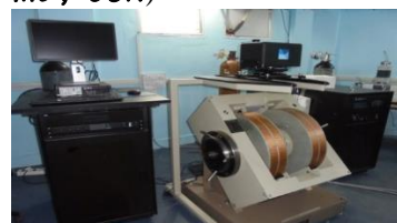
18. Vibrating Sample Magnetometer with temperature variation facility (Make: Lake Shore Cryotronics, Inc., USA )
