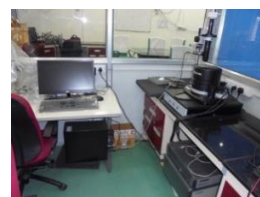
16. Impedance Analyser (40 Hz – 110 MHz) with temperature (up to 1000°C) variation facility. (Make: Keysight Technologies, USA)
