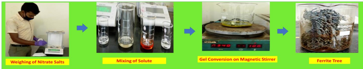
Flowchart of Preparation of Ferrite Magnetic Materials Tree in the Lab
