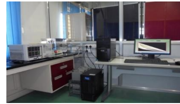
16. Impedance Analyser (40 Hz – 110 MHz) with temperature (up to 1000^\circ C ) variation facility. (Make: Keysight Technologies, USA)
