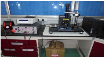
17. Precision Multiferroic Test System ( P-E , piezoelectric, pyroelectric, magneto-electric for bulk and thin-films) with temperature variation facility (Make: Radiant Technologies Inc., USA)
