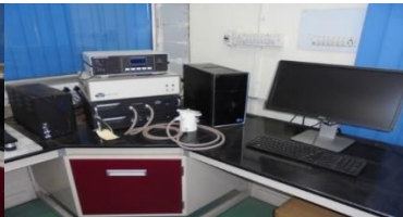
17. Precision Multiferroic Test System ( P-E , piezoelectric, pyroelectric, magneto-electric for bulk and thin-films) with temperature variation facility (Make: Radiant Technologies Inc., USA)
