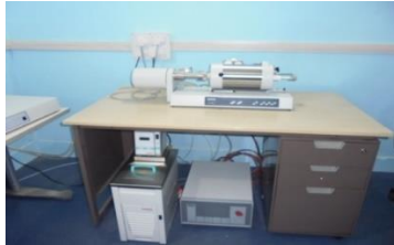
17. Precision Multiferroic Test System ( P-E , piezoelectric, pyroelectric, magneto-electric for bulk and thin-films) with temperature variation facility (Make: Radiant Technologies Inc., USA)
