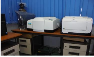
14. High Temperature ( lq. N_2 - 1600^\circ C ) Simultaneous TG-DTA / DSC Analyser (Make: NETZSCH Technologies, Germany )
