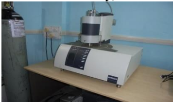
14. High Temperature ( lq. N_2 - 1600^\circ C ) Simultaneous TG-DTA / DSC Analyser (Make: NETZSCH Technologies, Germany )
