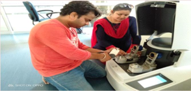
High Energy Ball Milling for Production of Nanomaterials;
