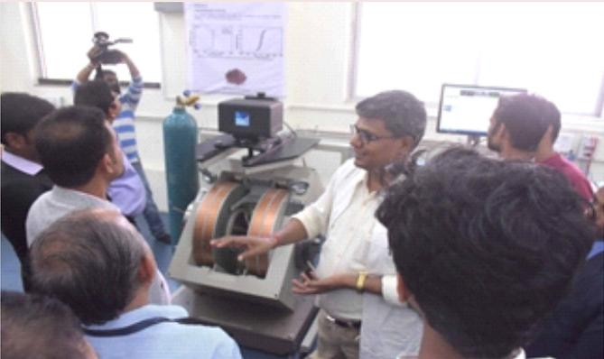
Vibrating Sample Magnetometer for Magnetic Measurement
