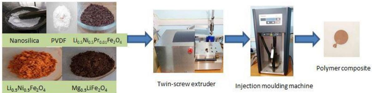
Materials used in the preparation of polymer composite
