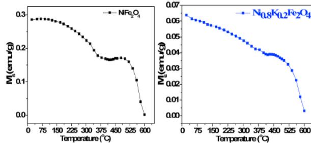
Fig. 12. Temperature-dependent saturation magnetization for  $NiFe_2O_4$  and  $Ni_{0.8}K_{0.2}Fe_2O_4$ .
