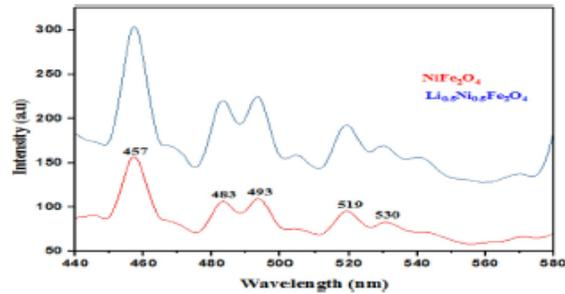
Fig. 9. Photoluminescence Spectra of  $\text{NiFe}_2\text{O}_4$  and  $\text{Li}_{0.5}\text{Ni}_{0.5}\text{Fe}_2\text{O}_4$ .
