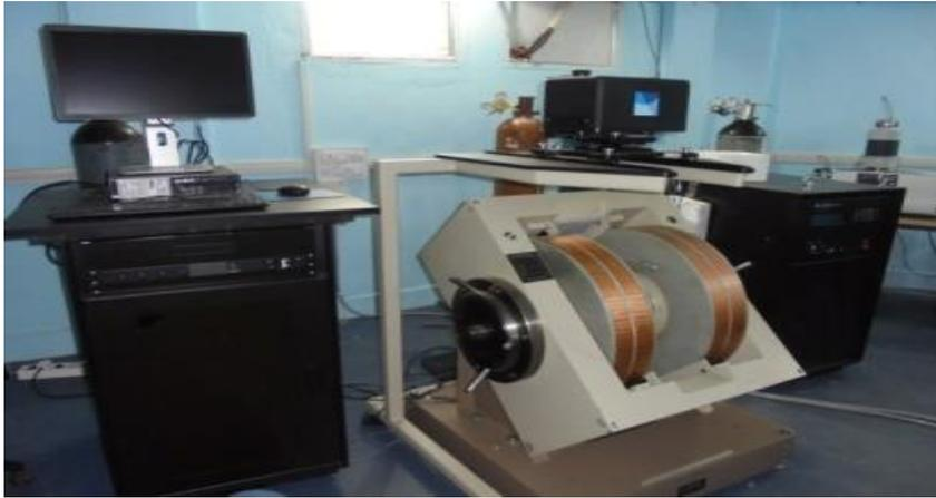
Vibrating Sample Magnetometer
