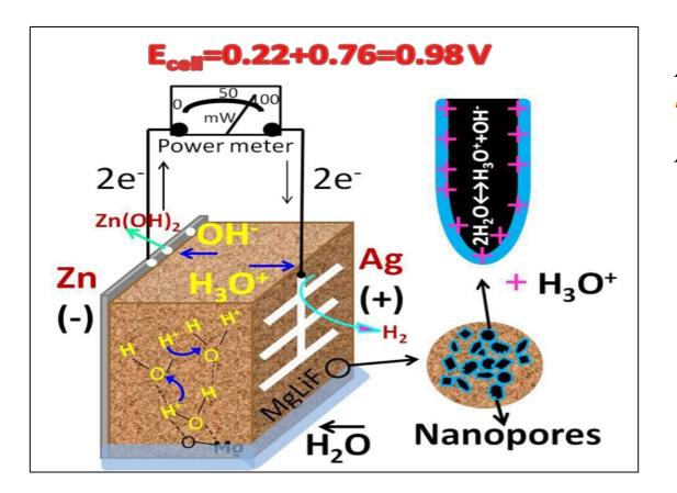
At Li-MgFe<sub>2</sub>O<sub>4</sub>:  $4H_2 O \rightarrow 2H_3 O^+ + 2OH^-$ At Zn electrode:  $Zn + 2OH^- \rightarrow Zn(OH)_2 + 2e^- E_{oxd} = -0.76V.$ At Ag electrode:  $2H_3 O^+ + 2e^- \rightarrow H_2^+ + 2H_2O$   $E_{red} = +0.22V.$ Total Cell Potential: 0.22V+0.76V = 0.98V
