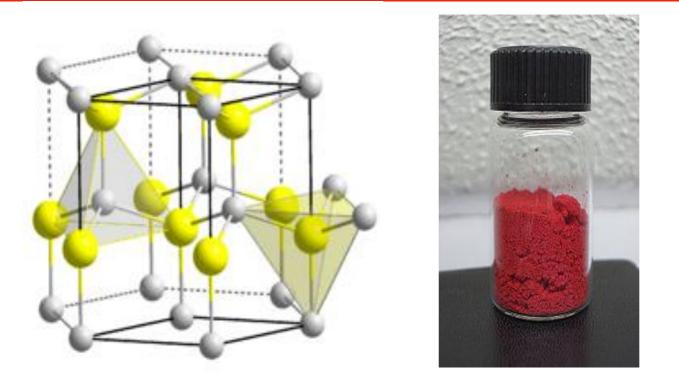
Cadmium Selenide quantum dots have been implemented in a wide range of applications including - Solar cells, Light emitting diodes, Biofluorescent tagging., CdSe-based materials also have potential uses in biomedical imaging, By injecting appropriately prepared CdSe nanoparticles into injured tissue, it may be possible to image the tissue in those injured areas and some others.
