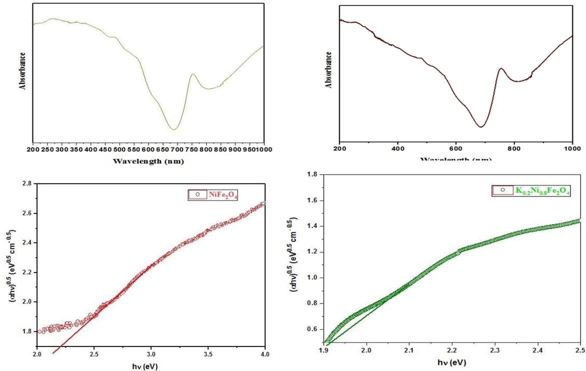
Fig. Tauc plot showing Indirect band gap of  $\text{NiFe}_2\text{O}_4$  and  $\text{Ni}_{0.8}\text{K}_{0.2}\text{Fe}_2\text{O}_4$
