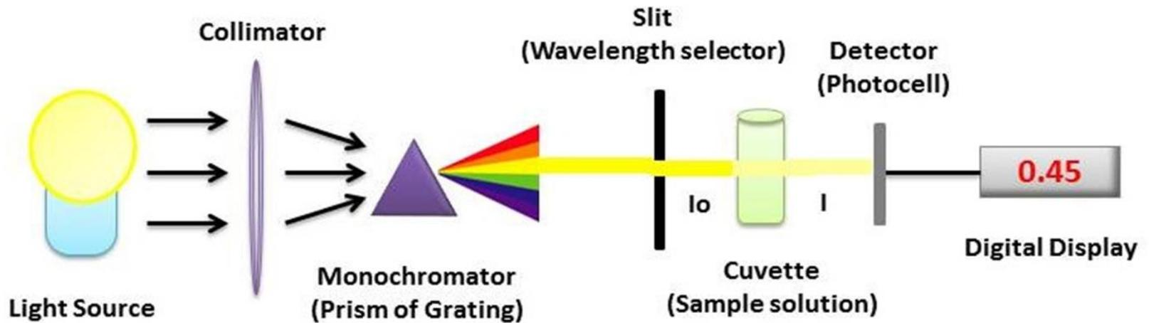
**Light source used Tungsten filament lamps and Hydrogen-Deuterium lamps.** **Filters.** **Interference filters:** use constructive and destructive interference to isolate a narrow beam of wavelengths. **Absorption filters:** Works by selectively absorbing radiation from a narrow region. Finally through prism and grating, monochromatic light allowed to pass to the materials.
