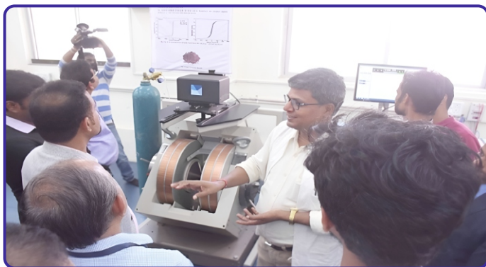
Vibrating Sample Magnetometer for Magnetic Measurement
