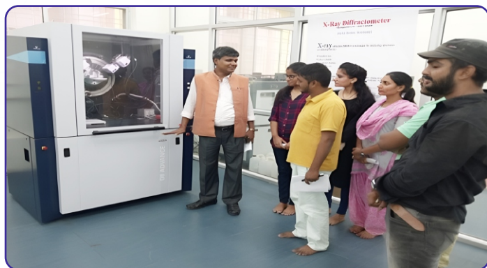
X-ray diffractometer for crystalline size/structure measurement
